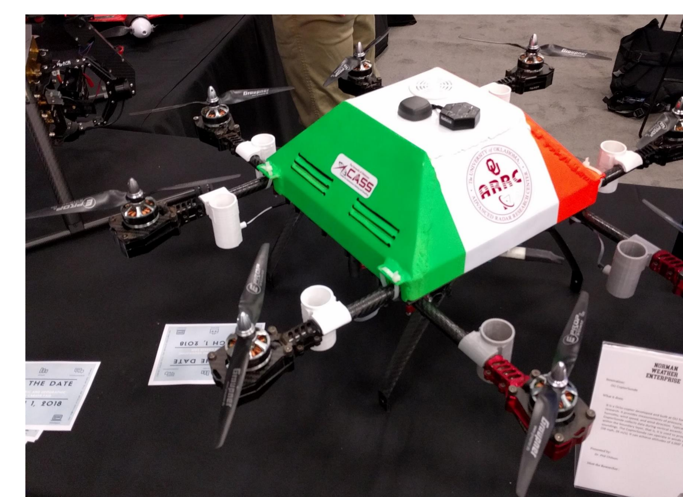
OU Coptersonde: Sensors integrated with Pixhawk
